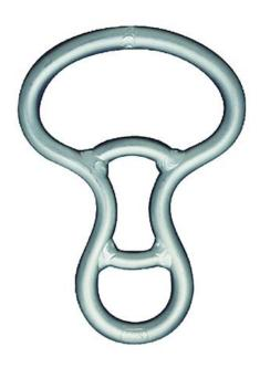
The Descent Control 8 provides exceptional control. This descender performs well in repetitive rappelling and descending environments. The unique shape prevents the un-weighted end of the rope from rubbing against the rope passing around the neck of the descender. As with all SMC products, welding is done by aircraft certified welders.
