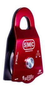
The unique shape of SMC's aluminum side plates allow the efficient use of Prusik hitches as a belay or progress capture device. Constructed with a 3" diameter sheave running on a high efficiency ball bearing. Low profile fasteners help eliminate the possibility of the pulley snagging. Pulley will accommodate up to 13 mm rope.
