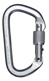
This carabiner sets the standard in climbing, mountaineering, and rescue applications. Extremely lightweight, it offers high strength and a large gate opening for functional versatility. The locking sleeve engages the gate rather than the frame to prevent jamming.
