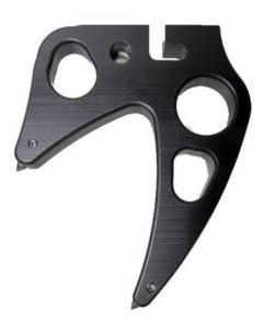
The TerrAdaptor<sup>™</sup> Talon Foot includes two spikes which allow the feet to be perched on edges of walls and catwalks, or they may also be lashed securely to pipes, beams, and rails. The steel tips of the foot may be sharpened or replaced.
