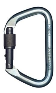
Large size locking carabiners developed by SMC especially for the needs of the fire and rescue communities. Available in several different metal finishes, as well as in both NFPA (Class G) and non-NFPA versions. Black zinc coated models are ideal for tactical operations and stainless steel model is best for corrosive environments. Large gate opening fits easily over litter rails. All models have stainless gates and locking sleeves for greater strength and reliability.
