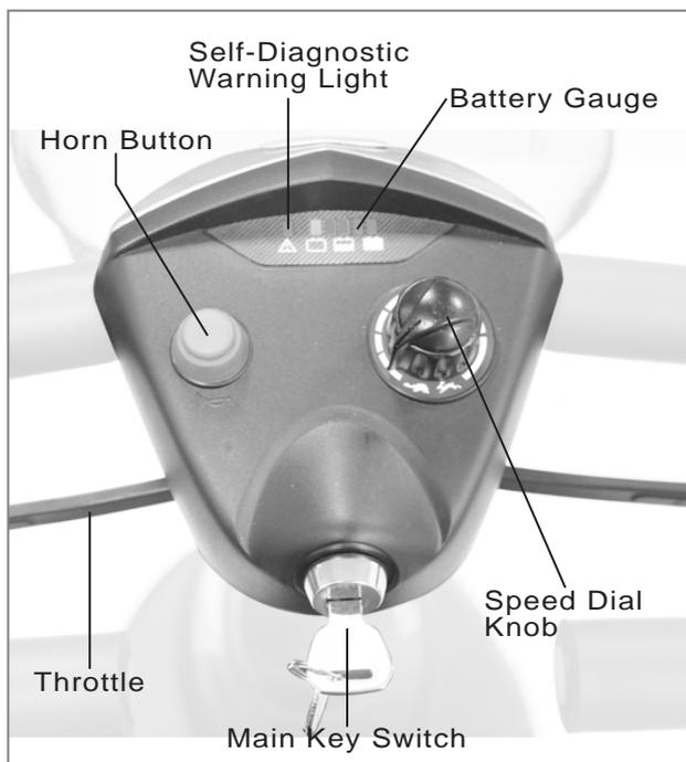
Figure 2 - EW-M39 Top Control Panel
