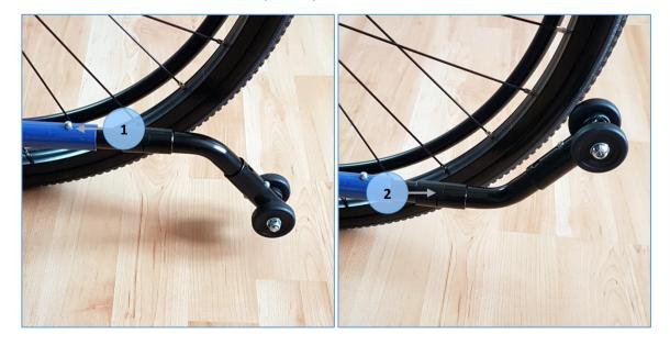
If the wheelchair is to go up or down a high step (e.g. a curb), the anti-tip wheels must be swiveled upwards to avoid them catching on the ground. Pull on them to unlock (2) and swivel up/down so it looks like picture 2 above.
