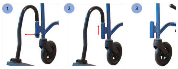
The plastic footrest tray can be adjusted in height to allow the user maximum comfort. The small bolt can be removed from the base of the plastic footrest tray and re-inserted into one of the three possible elevation holes on the footrest tube by using the Allen wrench provided with the wheelchair.
