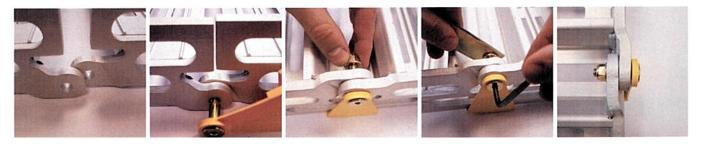
Use the 3/16" Hex Allen Wrench and a 1/2" wrench or the wrench provided. Align ramp sections - insert bolt through hole - tighten with Allen Wrench and wrench provided or a 1/2" socket. **Note:** Do **NOT** fully tighten nut to be able to roll up.
