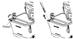
1. Insert the probe holder in the SmartBucket as shown in the illustration below.
