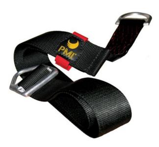
This traditional pick off strap has a metal D ring at the rescuers end for a metal-on-metal connection. Once connected, slack can be removed simply by pulling on the free end of the strap.
