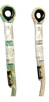
The Compact Sewn Termination for <u>11 mm PMI® Extreme Pro Rope</u> is available with either one or two ends. PMI uses precision stitching to create a permanent, sewn termination that is stronger than any knotted termination and nearly as strong as the rope itself. Heat shrink tubing protects the stitching and the label from abrasion.
