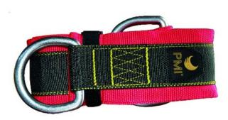
Wrapped around a beam, the new PMI® Choker sling provides a quick and safe anchor. An extra piece of webbing is sewn on the entire length of the sling to protect it from sharp edges and prolong its life.
