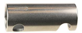
This 1" Tubular Stainless Steel Brake Bar features an angled slot. Using stainless steel means that the bar will last longer and will not leave the residual aluminum streaks on your rope like the aluminum alternatives. The angled slot helps keep bars still once it has been snapped in place.
