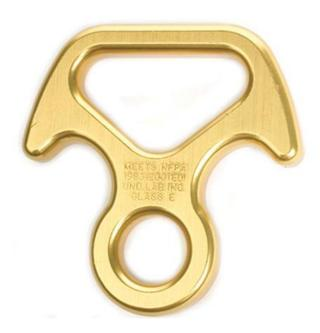
When easy application and removal of an escape descender is desired, the SMC Escape 8 is a convenient choice. Familiar figure 8 shape is modified and optimized for descending on small diameter ropes.
