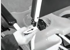
**28.** If the elevating or gooseneck leg rests were ordered, insert the ends (with the pin) into the receiver of the front support.
