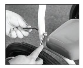
25. If the armrests were ordered, depress the snap buttons on the armrest assemblies and insert into the armrest pivots.
