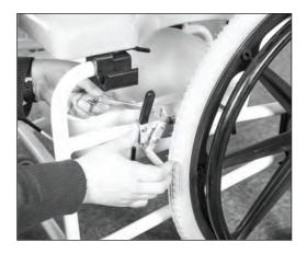
**22.** Loosen then remove the self-locking nut, plastic washer and machine screw that are in the chair frame where the back assembly will be attached.
