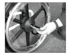
**16.** Place washer on bolt end to inside of wheel.
