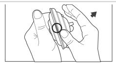
As shown in the picture, hold the top (smaller) case of the Back-flow Protector in one hand and place thumb of other hand on tab (circled) on bottom (larger) case. Pull the bottom (larger) case in the direction of the arrow to disassemble.
