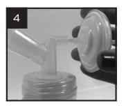
CONNECT the back-flow protector(s) to the top of the flange.
