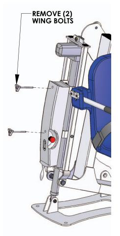
Remove the two (2) wing bolts connecting the control box to the bracket. Be sure to hold the control box as you remove the bolts to keep it from falling. See figure to the left.
