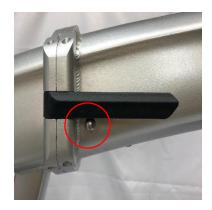
ground and then securely tighten front and back handlebar stem screws and check that the handlebar cannot rotate up or down. Each stem screw should be secured to the recommended torque value (16 nm/12 F-lb).
