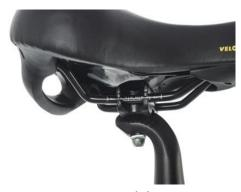
3. While holding the seat in the desired position, use a 6 mm hex wrench to tighten the seat adjustment bolt securely.
