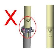
Ensure that the minimum insertion markings on the seat post are inside the seat tube of the frame (shown far right).
