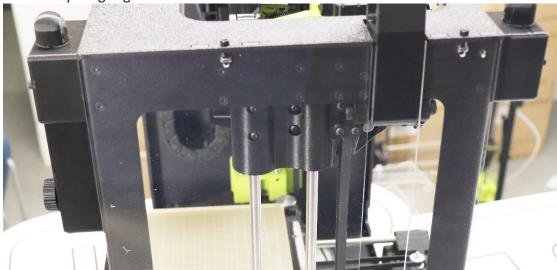
Using 2 M3-12mm bolts, square nuts and washer you can insert these from the outside with the nut and washer on the inside of the 2 diagonal slots at the bottom of the long side cover (Part J). The washer and nut help to hold the lower portion on the frame of the printer.
