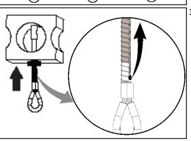
4. Pull on anchor loop and ensure toggle bar is fully seated in locked position as seen in the **TOGGLE POSITION DIAGRAM.** The hole plug should be fully seated in drilled hole.
