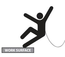
WARNING! Swing falls may occur when the worker is not directly under anchor point.
