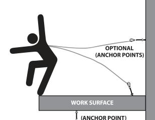
The user shall be equipped with a means of limiting the maximum dynamic forces exerted on the user during the arrest of a fall to a
