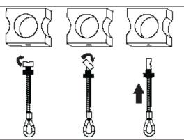
**3.** Push anchorage connector into drilled hole and engage toggle bar
