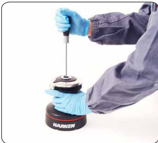
1. Unscrew the central screw ( \approx 2\text{Nm}/18\text{ in-lb} )
