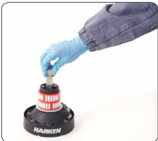
8. Slide out the central shaft n°19
