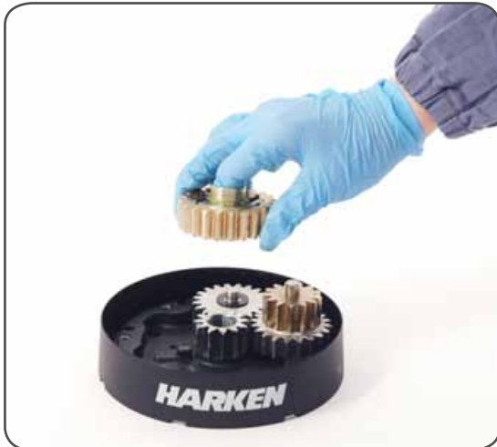
12. Remove the gear n°7 and remove the pawls n°5. To facilitate the operation press the spring against the pawl with a blade.
