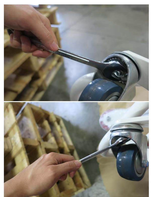
Turn the wrench counter clockwise (to the left) to loosen
