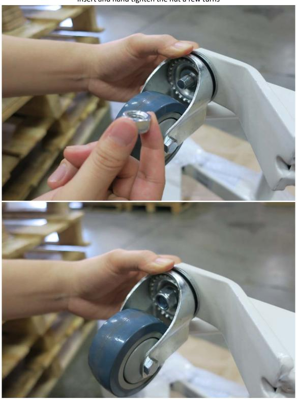
Turn the wrench clockwise (to the right) to tighten the nut all the way
