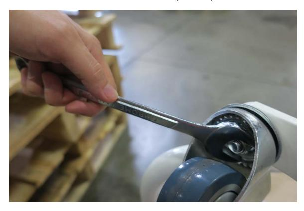
Once the nut is removed, remove the old caster.
