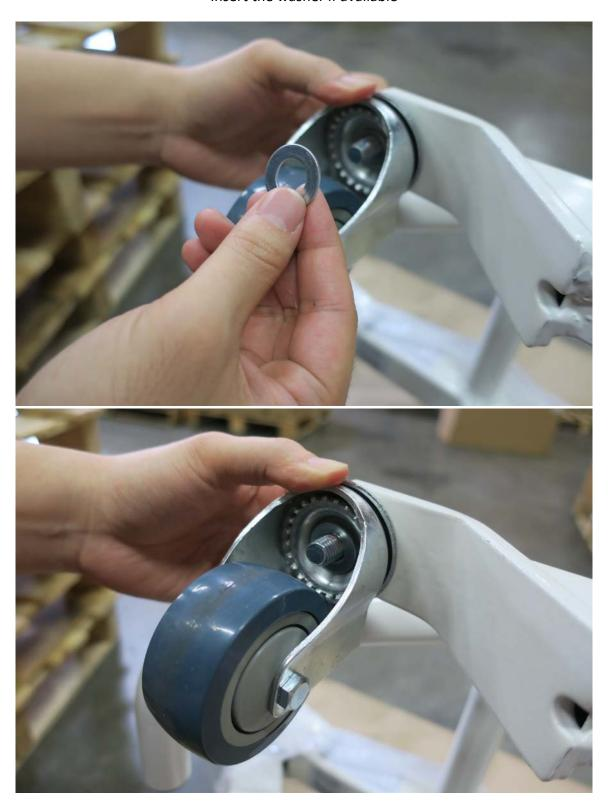
Insert and hand tighten the nut a few turns
