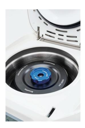
SCILOGEX rotors are manufactured from military-industrial grade aluminum alloy with high mechanical strength for precise running and safety (excludes SCI-12 rotor)
