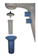
**Note:** It is recommended to check and clean the silicone adapter every six months, or when necessary, to prevent a loss of vacuum. If there is a loss of vacuum, please contact the manufacturer or your local distributor.
