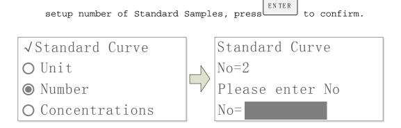
7) Calibrate Standard Samples.Put the corresponding standard samples in the light path as the screen indicates, input the concentration
