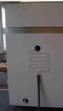
Insert the glas cooling coil through the hole on the left hand side of the prepASH into the centring lead.
