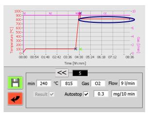
In step 5 you can change the ashing temperature and time. You are also able to set an autostop criteria. The result is taken automatically at the end of the step.
