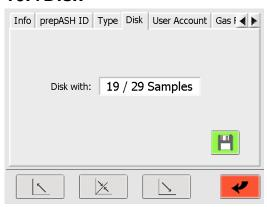
For the models prepASH229 and prepASH219 you can switch between the sample disks "19/29 Samples" and "12 Samples".
