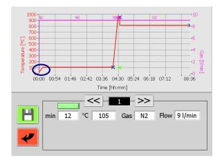
Step 1 is the ramp for the drying temperature. The ramp is limited to 50°C/min.
