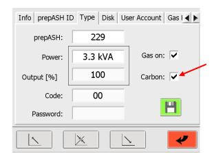
To use the carbon application, the function has to be activated in the service mode. Unlocking can only be made by a Precisa engineer.
