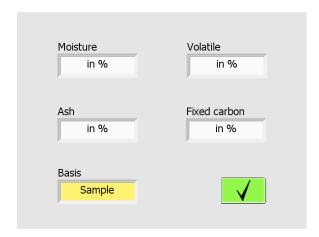
Before saving, you are asked for the calculation of the results. In every method will the moisture, volatile, ash and fixed carbon be calculated. You are able to choose showing the results in [%] or [g] and the basis of the calculation (sample or dry mass).
