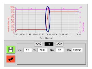
Step 3 is the ramp for the temperature where the volatile is taken.
