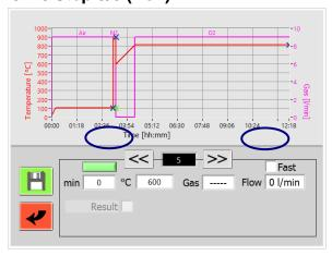
In step 5, you can enter the duration of the heating up to ashing temperature (from firmware release A1-1-2-04.)
