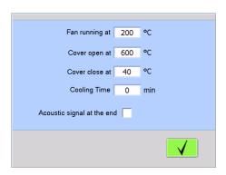
**Fan running at**: at temperatures above this temperature the exhaust is running and the lid is cooled. The fan has to be running before the decomposition of the organic compounds starts (Temp. < 200 °C).
