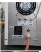
Connect the scrubber to the power outlet on the back side of the prepASH, see also chapter 2.4.2. Use the special Mains connection cable delivered with the scrubber connection set, 340-9002.
