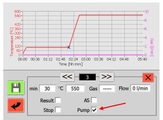
The scrubber is normally switched on during the ramp up to the higher temperature. Therefore activate the pump control in this phase only.
