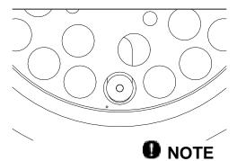
The small hole in the sample plate must lie to the left of the balance pan (refer to figure on the right)
