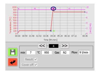
The time that you enter in step 4 is between achieving the temperature criteria (that is 2% under the set temperature) and the start of the volatile measurement.
