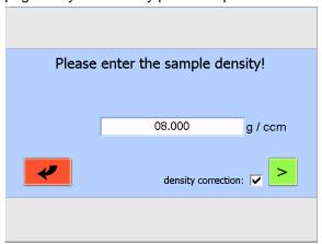
The entering of sample density is recommended for inorganic samples which have only a low loss on ignition and a large ash volume. The densities of these samples change only slightly during the analysis, the buoyancy change however is not negligible.
