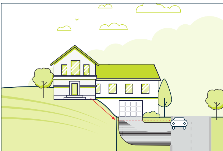
CROSS SLOPE ▶ change in slope that runs across the width of the ramp
