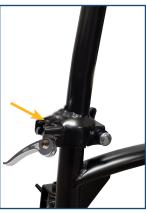
**2.** Slide locking mechanism into groove on tiller, depress locking handle to secure tiller lock.
